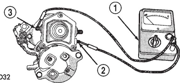
**Fig. 7 Continuity Test Between Solenoid Terminal and Field Coil Terminal - Typical**
