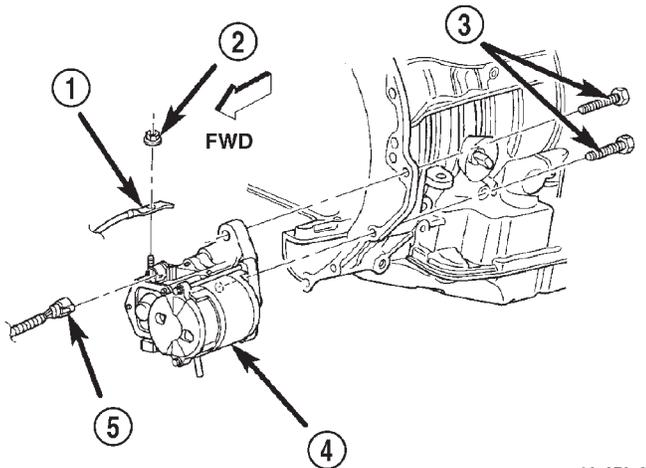
**Fig. 11 Starter Motor Remove/Install - 4.7L Engine**
