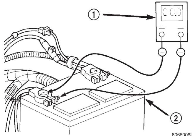
**Fig. 2 Test Battery Negative Connection Resistance - Typical**
